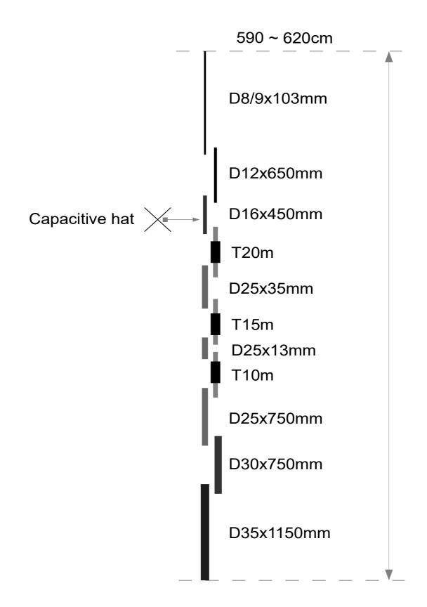
The antenna and solid radials length can change in according with tuning setting and/or possible environmental influences
