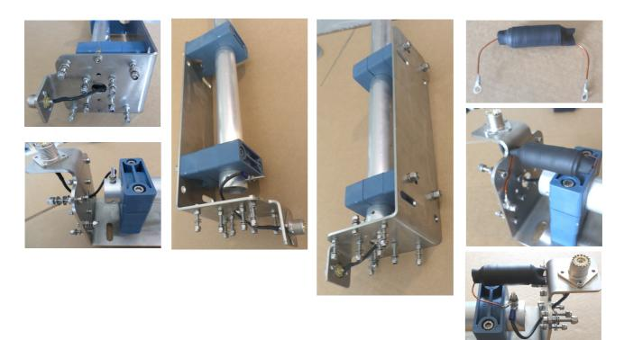
The care and precision of this assembly will ensure a long life to the antenna. Check that all bolts have been properly secured and completed the radiator assembly. With the aid of the U bolts, install the base on the supporting pole and install the solid radials. The U bolt is 50mm wide, it can get poles or tubes from 40 to 50mm.
