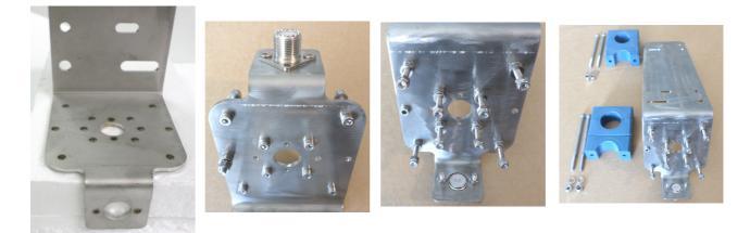
Install the 8 bolts 4x25MA in the holes in X shape and 4x16 bolt in the side hole as pictures. Correct assembling sequence for all the bolts: bolt, serrated washer, normal nut, two flat washers and self-locking nut. Block all tightening bolts thoroughly normal nut.
