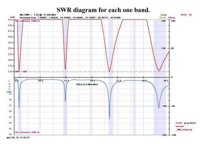
Note: The SWR curves, refer to an antenna installed at about 2m in height on draining soil, in semidry condition, free from obstacles in the immediate vicinity. The same curves are also valid for the version with wire radials installed a few cm from the ground on the same ground and in the same type of space.
